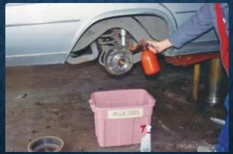
A mechanic removes asbestoscontaminated dust from brakes.
